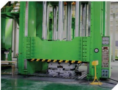
Press Molding Press SMC with GF mat under high temperature up to 150 °C and high pressure of min. 500~1500 tons.
