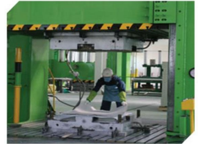
Placing Materials in Molds Charge the molds with materials (SMC and Glassfiber mat) according to designed patterns.
