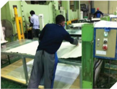
Cutting Sheet Molding Compound SMC, the mixture of unsaturated polyester resin, Glass fiber, filler, mold release agent and catalyzer
